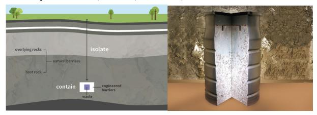
Providing safe, permanent disposal of legacy and future higher activity radioactive waste is essential. Deep burial of waste in a Geological Disposal Facility (GDF) is the internationally recognised preferred way forward.
